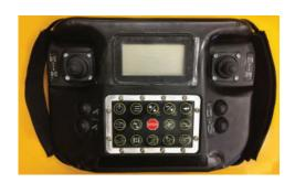
**CONVENIENT CONTROL.** The transceiver remote is equipped with a fault log, machine control menu, and the ability to supply the user with machine-operating information to monitor the machine's health.
