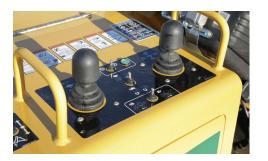
**OPERATOR PRESENCE SYSTEM.** The dual-axis joystick control handles for boom swing, boom raise/lower and machine propel are equipped with an operator presence feature. This user-friendly operator presence system is intended to enhance operator safety.
