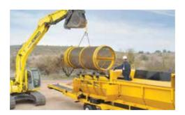
**SERVICEABILITY.** Removable side panels make drum removal efficient and provide convenient access for maintenance and cleaning.
