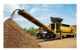
**QUALITY OUTPUT.** Designed specifically to process topsoil with high moisture content while maintaining a consistent, quality output — up to 150 cu yd (114.7 m³) of material per hour.
