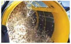
**HIGH PRODUCTION.** The tensioned screens around the drum add rigidity, allowing use of smaller-gauge wire — helping increase production capacity and enable processing of wetter material.
