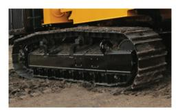
JOBSITE MOBILITY. Efficiently move the machine around jobsites without the need for for additional support equipment. The undercarriage offers 29 inches (73.7 cm) of belly clearance and rising chain rollers for material cleanout.
