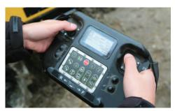
**CONVENIENT REMOTE CONTROL.** ACS control system designed specifically for this machine allows operators to engage/disengage the clutch, reposition the machine, adjust the discharge chute, and monitor the machine's health.
