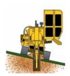
**OPTIONAL AUTO TILT TRACK.** An oscillating track frame allows the track to follow the ground's contour providing a vertical trench on slopes up to 10 degrees.
