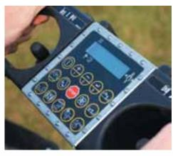
State-of-the-art wireless remote control units allow the operator to run most machine functions away from the machine. Remote controls are nontethered with a maximum working range up to 300' (91.4 m).
