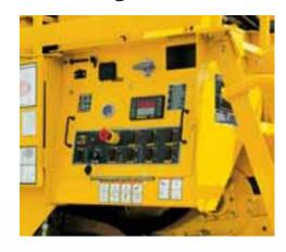
The standard microprocessorcontrolled HPTO clutch is designed to control the starting sequence with the push of a button — no need to bump a clutch. Minimal operator interface is required to initiate the grinding process.
