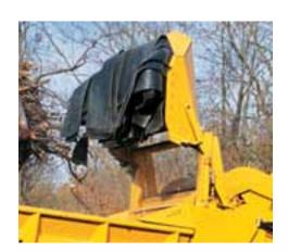
The innovative HG6000 / HG6000TX features the Thrown Object **Deflector (TOD).** The TOD reduces the quantity and distance of thrown material debris. Additionally, the TOD is strategically positioned to reduce interference when loading over-length material.
